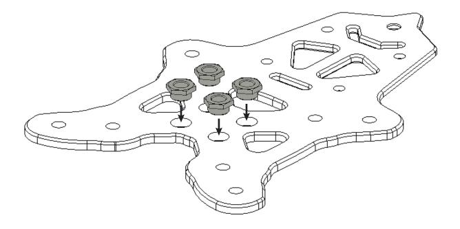
USE A BIG SCREW TO INSERT THE PRESSNUTS ONE BY ONE
